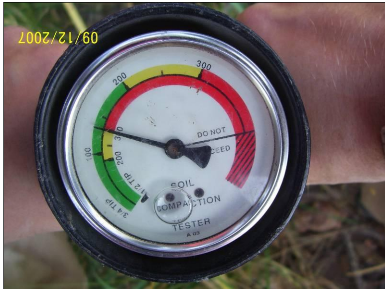
FIGURE 18. A CONE PENETROMETER DIAL, SHOWING PRESSURE APPLIED IN POUNDS PER SQUARE INCH.
