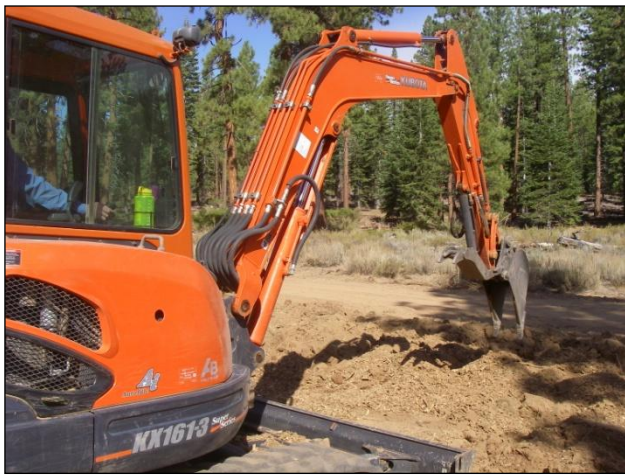
Figure 3. Ripping with the modified excavator bucket on plot 1.
