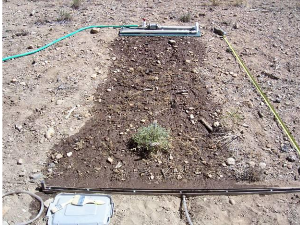
FIGURE 14. THE RUNOFF SIMULATOR AND PLOT. THE WATER DISPERSER IS AT THE TOP OF THE PHOTO AND THE COLLECTION FRAME IS AT THE BOTTOM.
