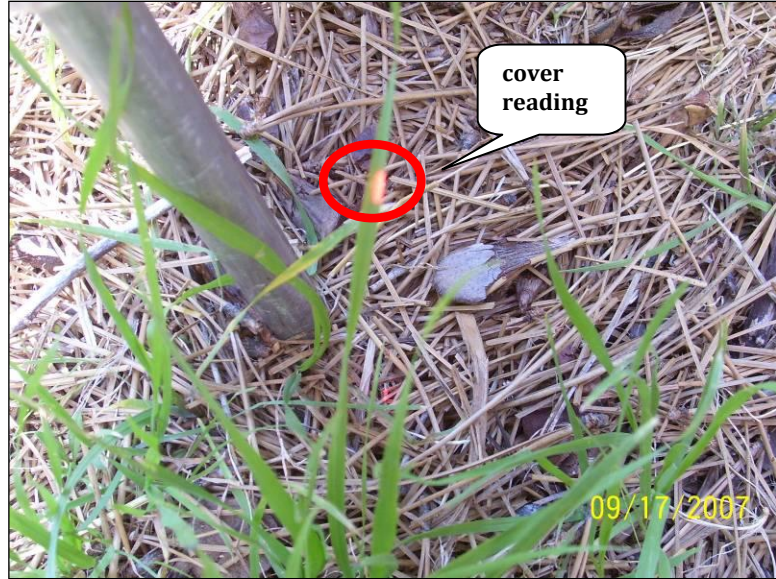
FIGURE 17. COVER POINTER ROD WITH HIT BY THE LASER POINTER. THE LASER POINTER HIT IS CIRCLED IN RED.
