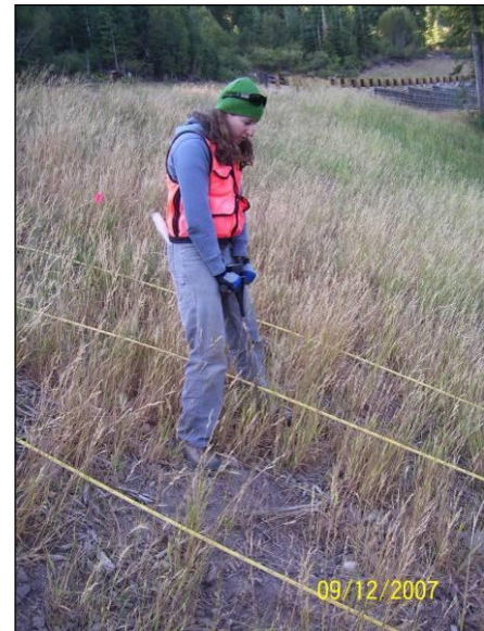
FIGURE 19. CONDUCTING CONE PENETROMETER MEASUREMENTS ALONG TRANSECTS.
