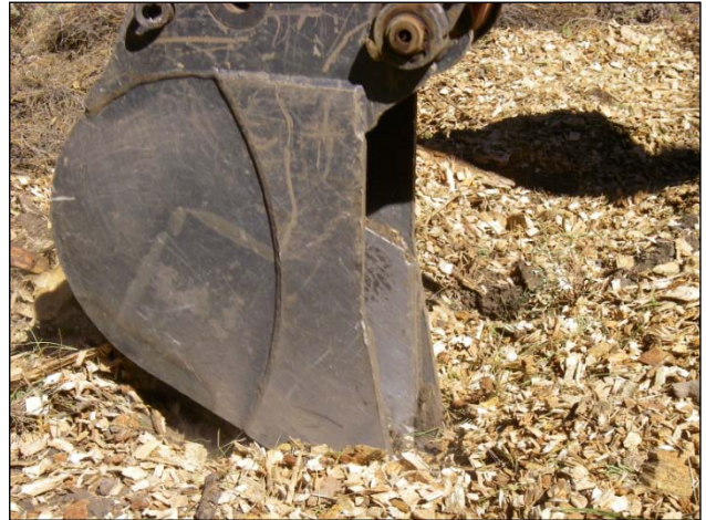
FIGURE 4. MODIFIED EXCAVATOR BUCKET RETRACTING FROM "TARGETED LOOSENING" WITHOUT TURNING SOIL.
